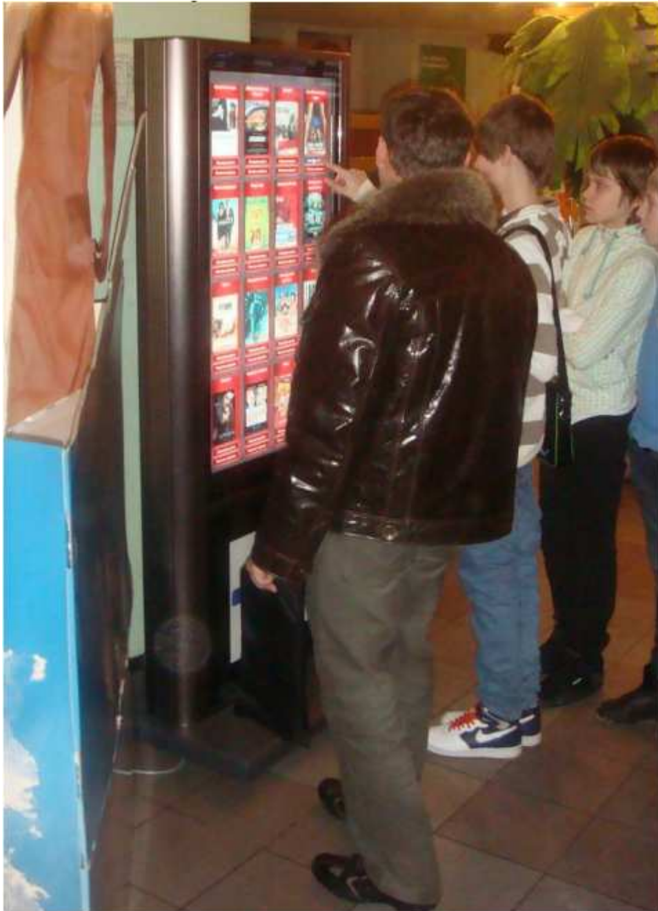
Foil on glass built into a totem with LCD behind
